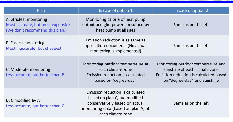
New Mechanism FS for Energy Saving at Buildings by Utilising Geothermal Heat Pump and Other Technologies in Mongolia
