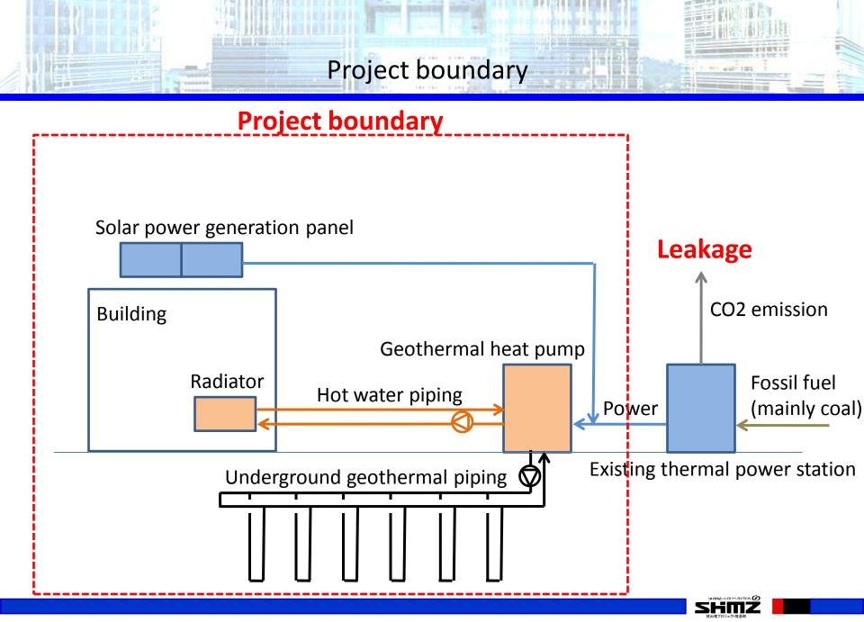
New Mechanism FS for Energy Saving at Buildings by Utilising Geothermal Heat Pump and Other Technologies in Mongolia
